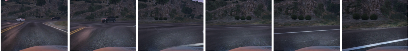
Figure 18: Some video sequences showing the evaluated model driving in the GTA V simulator. We show some difficult cases: road covered by shadows (top), roads with vague lane markings, e.g. a bridge (middle), and a dark three-way crossing (bottom). Please refer to the supplementary material for the video version of these sequences.
