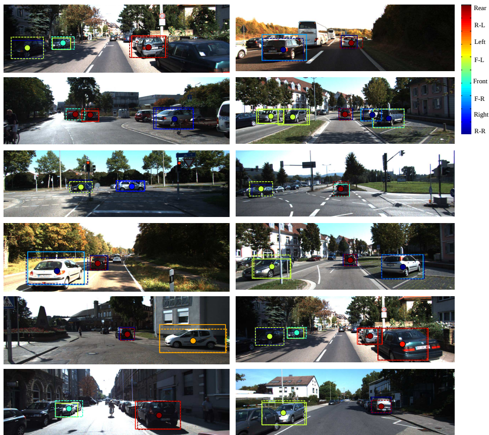
Figure 5.3: Viewpoint classification results encoded in jet scale. Continuous line, local detector prediction; Dashed line, scene-driven object proposals. Circle, ground-truth viewpoint. (Best viewed in color).
