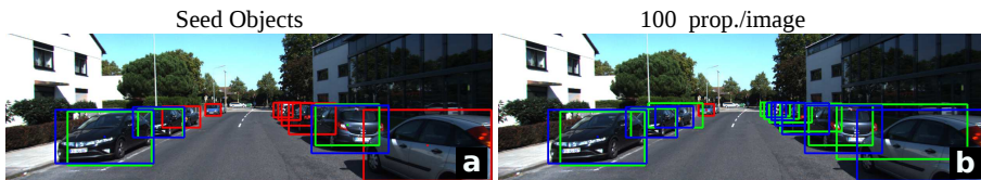
Figure 6.1: Object detections collected: a) after running a standard appearance-based detector, b) after sampling only 100 context-based object proposals post detection. Notice how we manage to recover many of the initial missed detections. For the sake of clarity in the visualization, we removed the false positive proposals and only show the bounding boxes of the matched object annotations (in blue), missed detections (in red) and matching object proposals (in green). (Best viewed in color).
