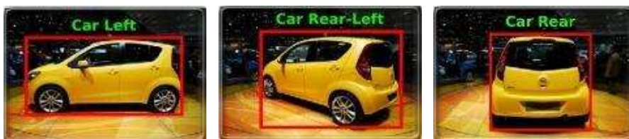
Figure 1.3: Car viewpoint estimation output. Note how in addition to the bounding box, a label indicating the predicted viewpoint is returned.
