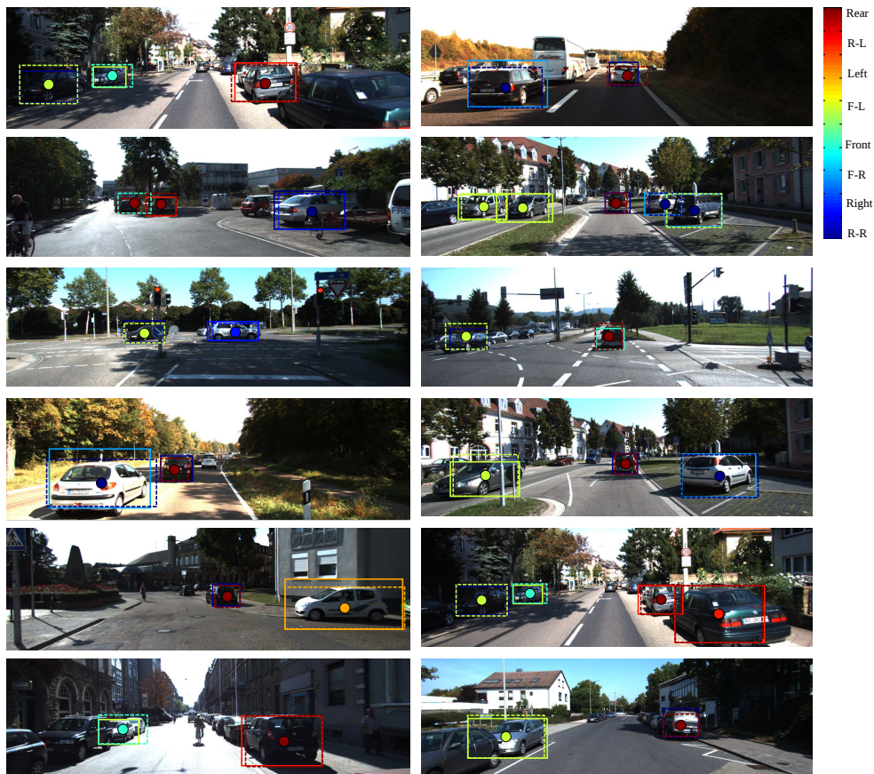
Figure 1: Viewpoint classification results encoded in jet scale. Continuous line, local detector prediction; Dashed line, scene-driven object proposals. Circle, ground-truth viewpoint.(Best viewed in color).
